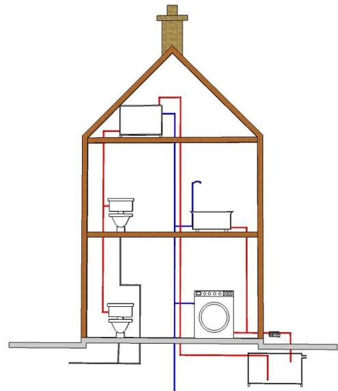
*A simple greywater system uses the outflow from showers, bathroom sinks and washing machines for flushing of toilets or outdoor irrigation*
