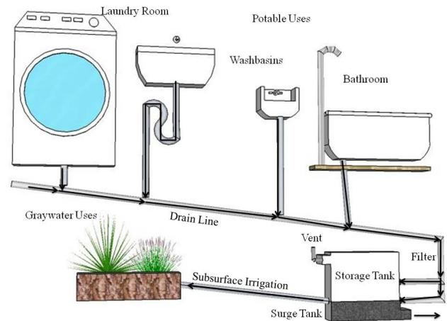
*A legal greywater system in Utah is only allowed to use the water for sub-surface irrigation purposes*
