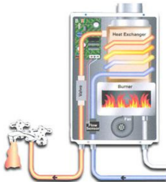
As cold water flows through the heating component the water is heated supplying a continuous flow of hot water instantaneously
